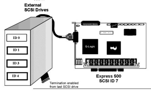
**Terminating Internal and External Disk Arrays** You can use both internal and external drives with MegaRAID Express 500. You still must make sure that the proper SCSI termination and termination power is preserved, as shown below:
